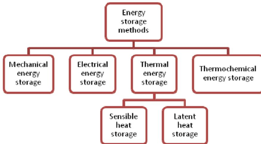
**Figure 1 Different types of energy storage methods [4].**
