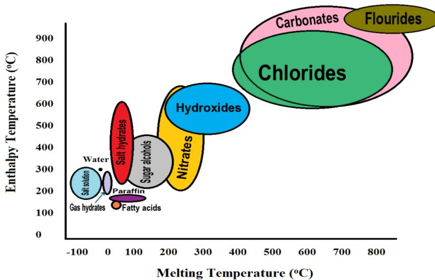
Figure 3. The typical range of melting temperature and enthalpy of PCMs [40]
