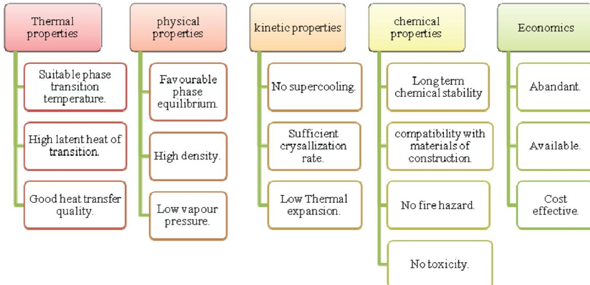
**Figure 3. Desirable properties of PCMs [5].**
