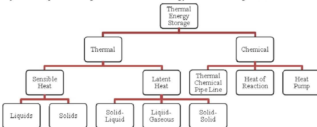
**Figure 2. Different types of thermal storage of solar energy [4].**
