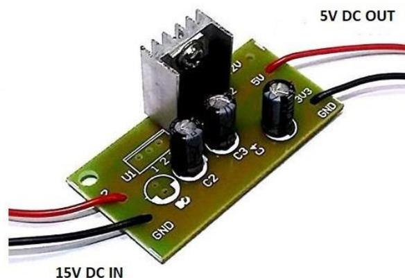
A voltage regulator is a circuit that creates and maintains a fixed output voltage, irrespective of changes to the input voltage or load conditions. Voltage regulators (VRs) keep the voltages from a power supply within a range that is compatible with the other electrical components. The presence of the two 100  $\mu\text{F}$  Capacitors is used to cancel out any kind of ripple present from the constant 5V output that comes out of the 7805 voltage regulators.
