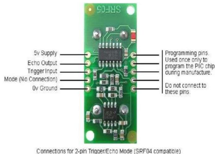
**Fig 2.1** diagram show the pin diagram and I/O ports of an Ultrasonic sensor
