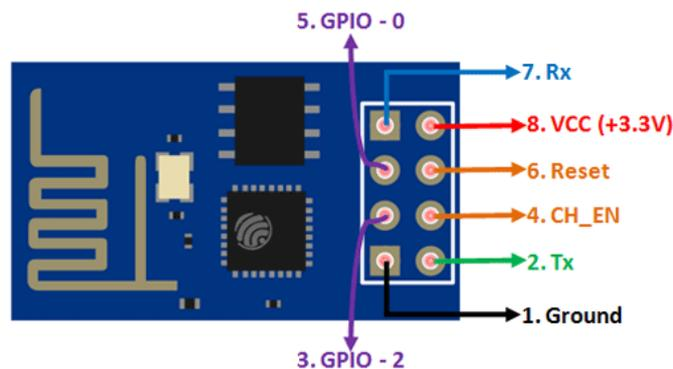
Fig 2.3 in out of the Wi-Fi module
