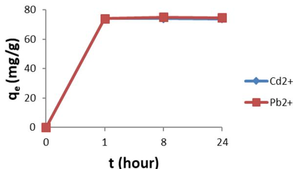
**Figure 10.** Cd<sup>2+</sup> & Pb<sup>2+</sup> biosorption of sorbent at 45°C, 75mg.L<sup>-1</sup> concentration & >0.5mm particle size (N=3)
