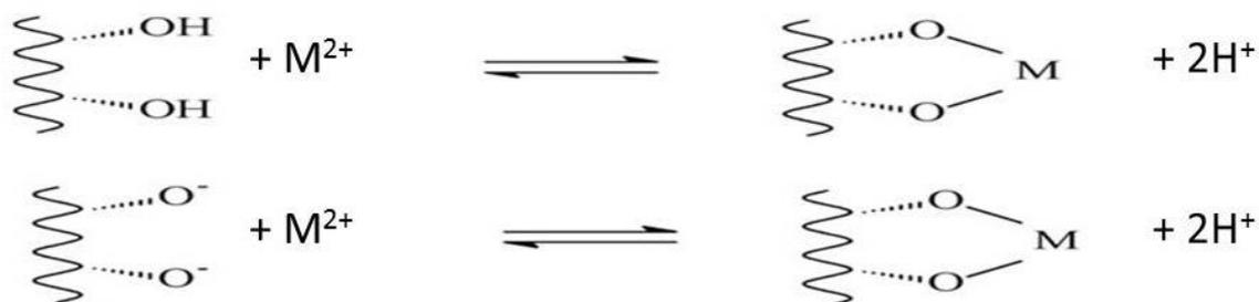
**Figure 11.** Mechanism of metal ions attachment to sorbent surface (Demirbaş et al., 2008)
