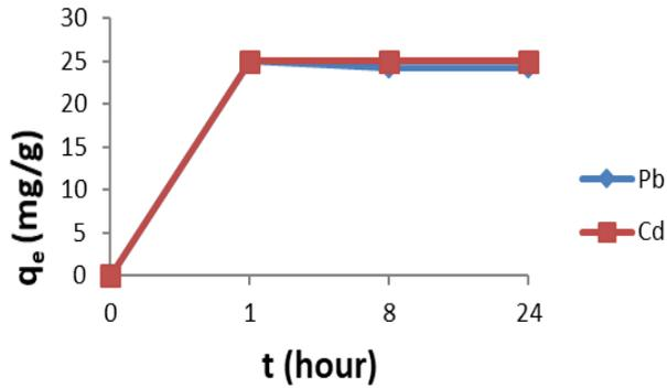
**Figure 6.** Cd<sup>2+</sup> & Pb<sup>2+</sup> biosorption of sorbent at 45°C, 25mg.L<sup>-1</sup> concentration & >0.5mm particle size (N=3)
