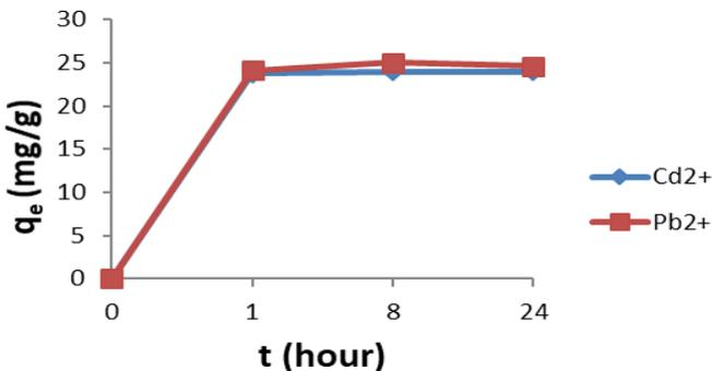
Figure 5. Cd<sup>2+</sup> & Pb<sup>2+</sup> biosorption of sorbent at 45°C, 25mg.L<sup>-1</sup> concentration &  $\le 0.5\text{mm}$  particle size (N=3)
