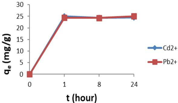
Figure 3. Cd<sup>2+</sup> & Pb<sup>2+</sup> biosorption of sorbent at 25°C, 25mg.L<sup>-1</sup> concentration &  $\le 0.5\text{mm}$  particle size (N=3)
