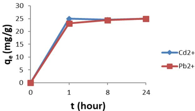
Figure 4. Cd<sup>2+</sup> & Pb<sup>2+</sup> biosorption of sorbent at 25°C, 25mg.L<sup>-1</sup> concentration &  $>0.5\text{mm}$  particle size (N=3)
