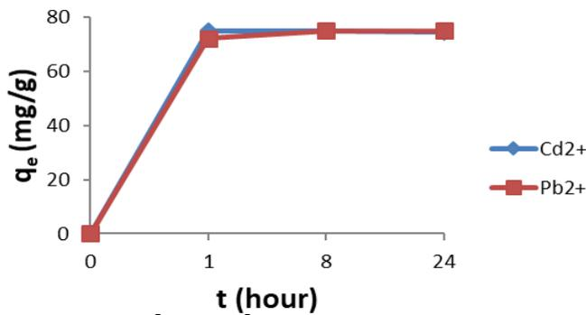
**Figure 8.** Cd<sup>2+</sup> & Pb<sup>2+</sup> biosorption of sorbent at 25°C, 75mg.L<sup>-1</sup> concentration & >0.5mm particle size (N=3)
