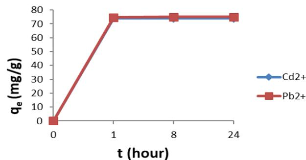
**Figure 9.** Cd<sup>2+</sup> & Pb<sup>2+</sup> biosorption of sorbent at 45°C, 75mg.L<sup>-1</sup> concentration & ≤0.5mm particle size (N=3)
