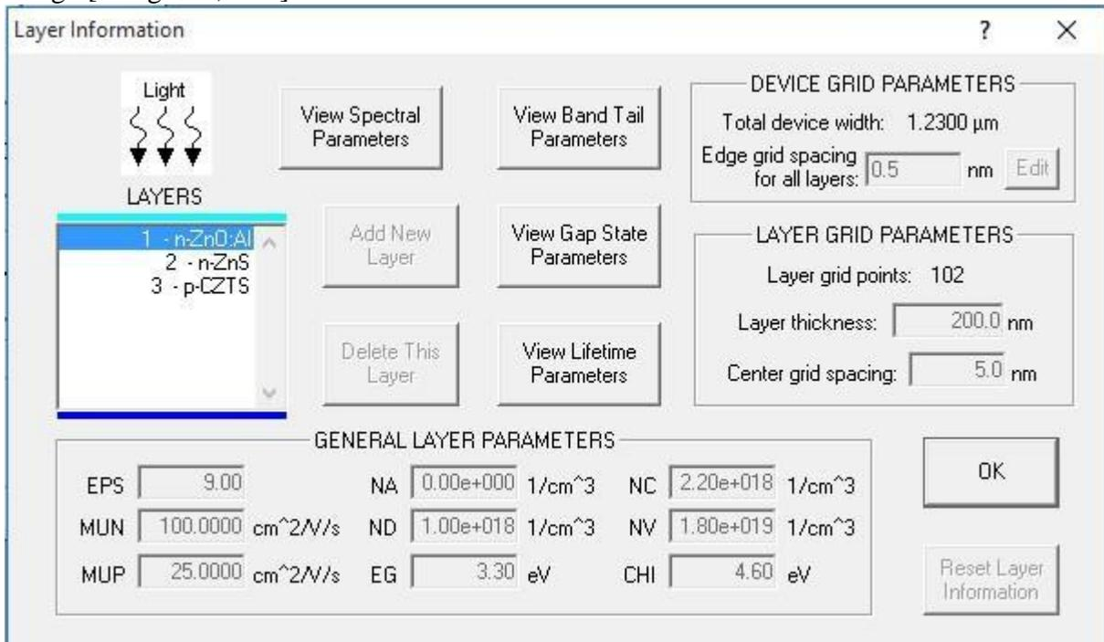
Figure 2: AMPS-1D simulation front panel contains the device and layer grid parameters, and general layer parameters
