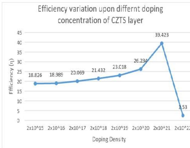
Figure -5: Efficiency and doping profile variation of CZTS absorber layer.
