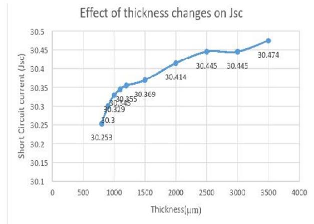
Figure -4(b): Short circuit current (Jsc) variation due to the change of absorber layer thickness
