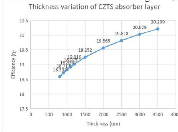
Figure 4-a: Efficiency variation due to the change of absorber layer thickness
