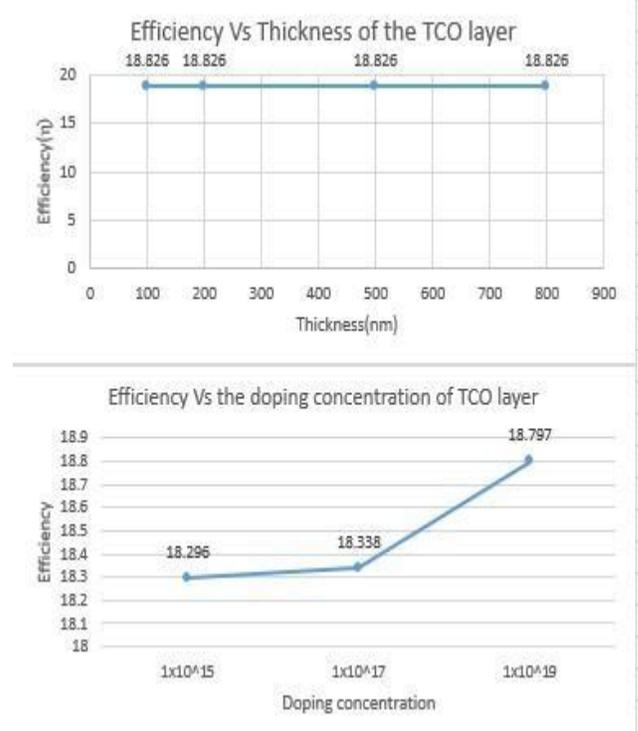
Figure-8: TCO layer Thickness and Carrier Concentration effect on overall efficiency of the cell
