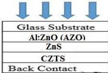
Figure -3: Simulated structure of AZO/ZnS/CZTS Solar Cell
