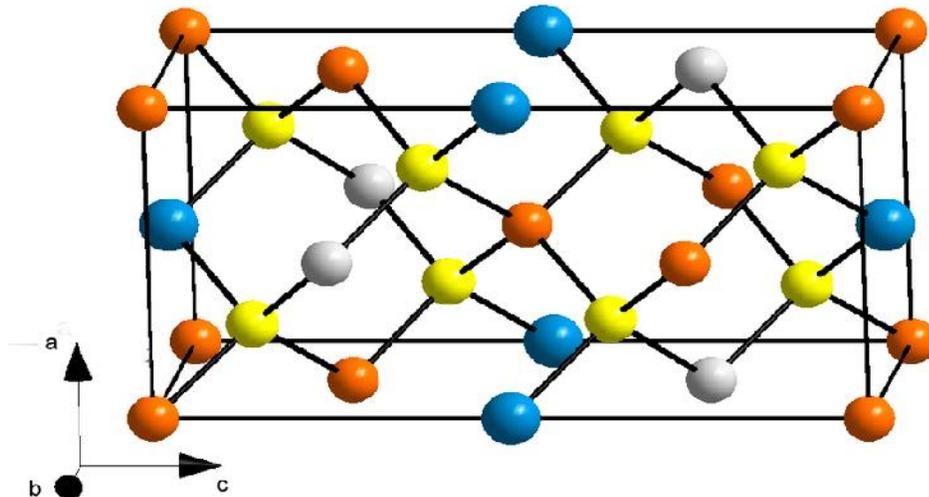
Figure 1: CZTS crystal structure. Orange: Cu, grey: Zn/Fe, blue: Sn, yellow: S.
