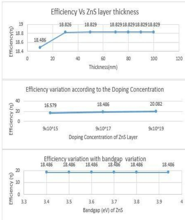
Figure- 7: Efficiency variation due to the changes of different material parameters of ZnS as window layer
