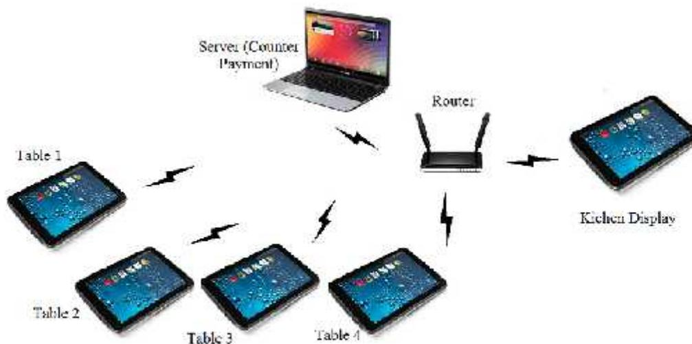
**Fig. 1 System Architecture**
