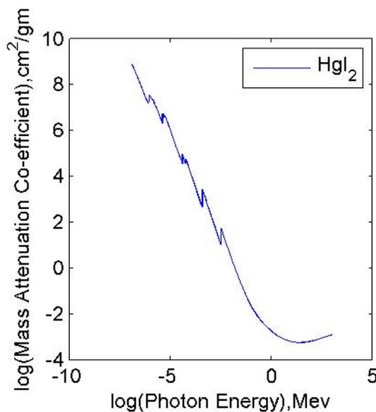
**Fig 1.** Mass Attenuation co-efficient vs Photon Energy for  $\text{HgI}_2$  in the energy range 1KeV to 20 MeV.
