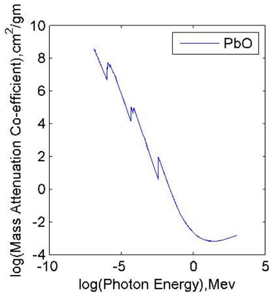
Fig 3. Mass Attenuation co-efficient vs Photon Energy for PbO in the energy range 1KeV to 20 MeV.
