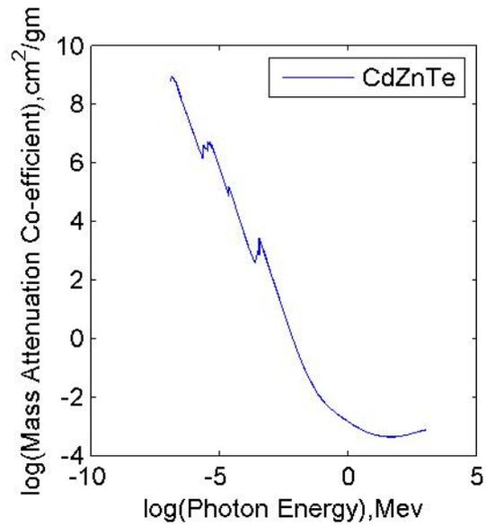
Fig 4. Mass Attenuation co-efficient vs Photon Energy for CdZnTe in the energy range 1KeV to 20 MeV.
