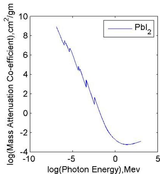
**Fig 2.** Mass Attenuation co-efficient vs Photon Energy for  $\text{PbI}_2$  in the energy range 1KeV to 20 MeV.
