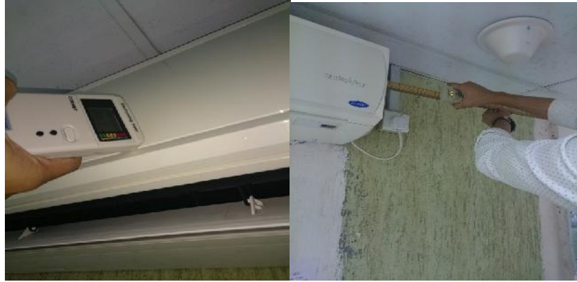
Figure 1: Electromog RF/LF Field Strength power meter Dual mode RF power meter & LF gauss meter ED-78S measuring magnetic field in front of air conditioner (left image) and the COGHILL FIELD MOUSE measuring the EF and MF threshold values (see green lights). Green lights indicate the EF and MF both threshold have reached. (Right image).
